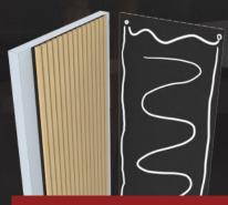
Attach acoustic panels to the wall with nail-free glue.
