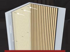
Nail acoustic panels directly to the wall.
