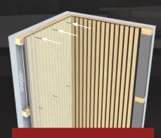
Install fibreglass wool or rock wool between the battens.
